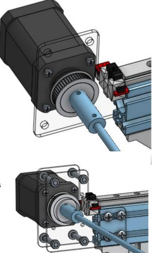
Then add the second bracket with the 4 bolts and the spacer between the brackets. Finally add the 5 mm screws to the T - Nuts in the Y axis.
