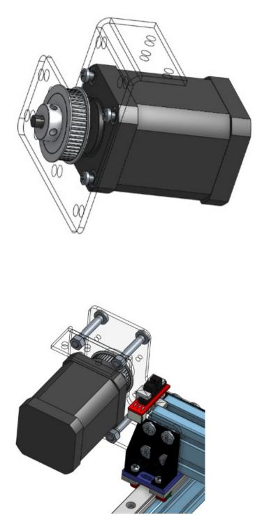
Here you put 4 M5 x 6mm through the bracket and into the 4 M5 T Nuts. Also use 2 M3 x 12mm screws down in to the slider bracket and attach it with 2 M3 nuts.
