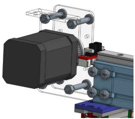
Now just like the idlers, you need to put the 4 M5 x 6 screws through the bracket and into the 5 mm T nuts. The T-nuts can be seen on this view.
